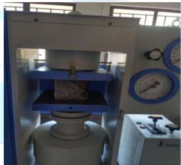
Figure 3: cube test under CTM
