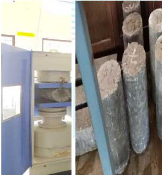
Figure 4: Cylinders testing under CTM
