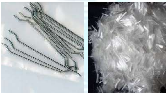
Figure 1: Hooked End Steel Fibres And Polypropylene Fibres
